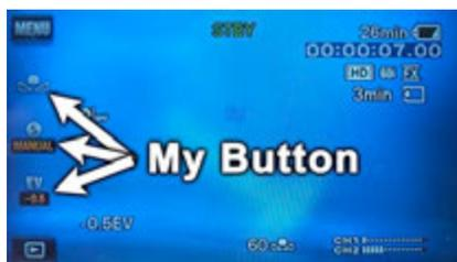
My Buttons provide quick access to frequently used adjustments such as White Balance, Gain, and “EV” (AE Shift – Automatic Exposure Shift). The buttons appear on the left side of the LCD screen when you cycle through the Display mode.
