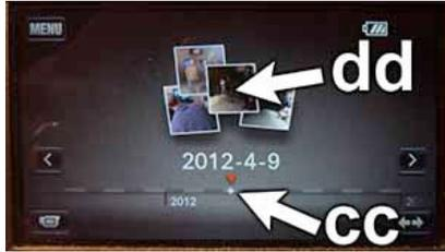
Put the camera into video playback mode. Scroll the time line (cc) near the bottom of the screen to select the video clips by date. Touch the clips above the date (dd) to bring up a grid of the clips.
